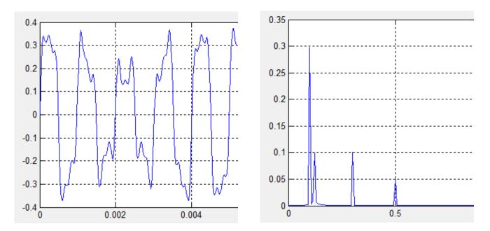
By dragging the **signal duration** slider, total amount of points in the signal is changed. This affects the DFT algorithm used to generate the spectrum, and because of that you can see how *spectrum precision is changed with signal duration*.
