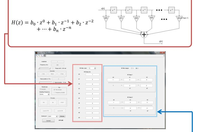
**Infinite impulse response** filter is implemented in the form of *Biquadratic cascade* filter. It consists of cascaded 2<sup>nd</sup> order stages with 3 feed-forward and 2 feedback coefficients each.
