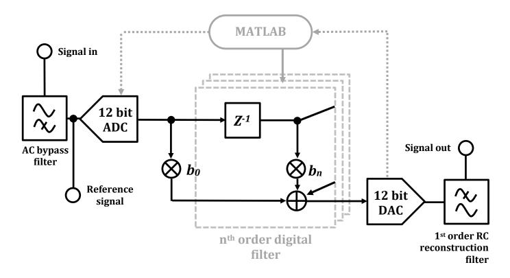
Prior to sampling, input signal is preconditioned with zero offset 10 Hz high-pass filter and biased for an ADC input. Sampled signal is processed with algorithm one sample at a time; delay line is updated each step. Reconstruction is done with customizable low-pass filter.
